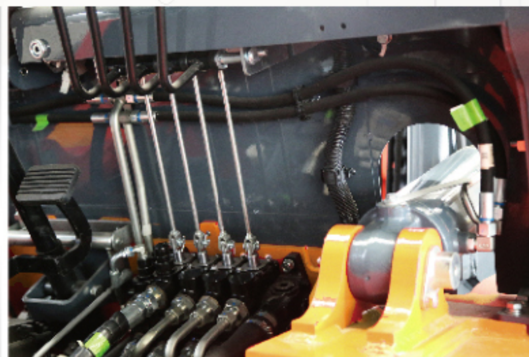
Large diameter hydraulic pipe, Standard 24 degrees conical seal.
