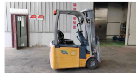
Cold storage test The whole truck was operated alternately in a -20 °C cold storage for 6 hours, and parked in the cold storage for 12 hours. The whole truck has no faults and could operate continuously
