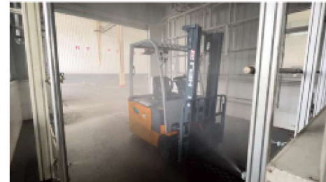
Rain test the truck reaches to IPX4 protection level after simulating operation under 15 min rainstorm and it meets outdoor operation requirements.
