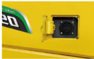
National standard fast charging port supports up to 200A fast charging
