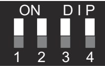
Figure 2-12: Board ID SW1 DIP Switch
