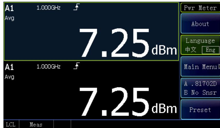
When the peak power sensor is connected, it becomes high-performance peak power meter. The amplitude and time domain parameters of pulse modulated signals in 50MHz ~ 67GHz band can be measured and analyzed.
