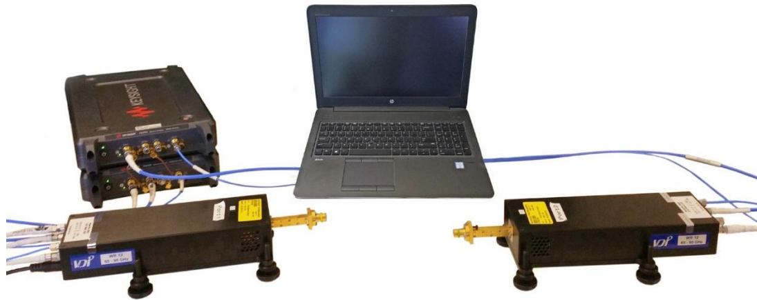
Figure 6. P9375A Streamline USB VNA based E-band VNA setup
