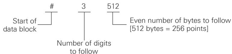
The instrument represents binary data as 16-bit integers, which are sent as two bytes. Therefore, the total number of bytes is always twice the number of data points in the waveform and must always be an even number. For example, 512 bytes are required to download a waveform with 256 points.
