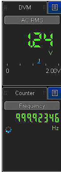
Figure 30. DVM and counter takes advantage of separate signal paths to provide measurements without a trigger, while still using the scope probes.
