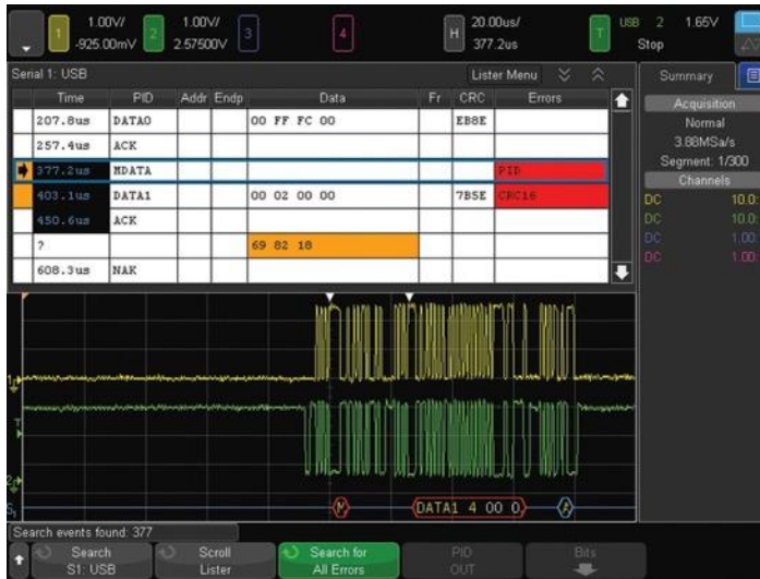
Figure 21. USB 2.0 trigger, decode and "lister" display.
