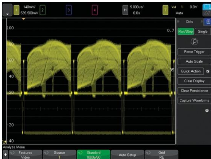
Figure 27. Triggering on 1080p HDTV signal analysis.
