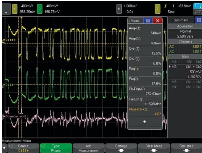
Figure 24. Dual channel WaveGen output of differential arbitrary signals. Common mode is shown as a math.
