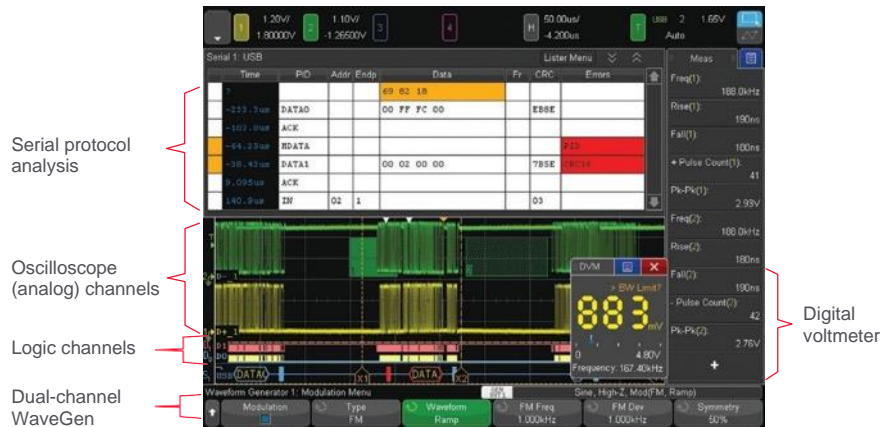
Figure 17. The 4000 X-Series provides the capabilities of seven instruments seamlessly integrated into one.
