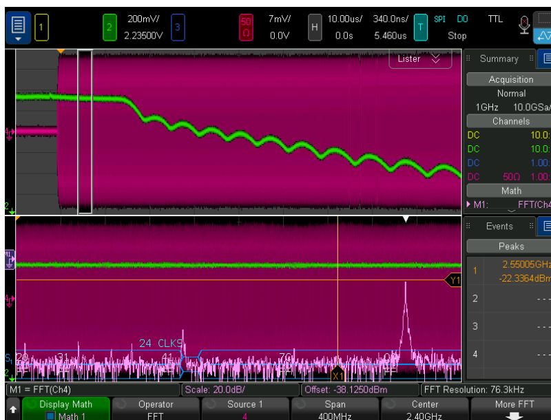
Figure 37a. Gated FFT time correlating the PLL voltage, SPI command and spectrum content at a given time span.
