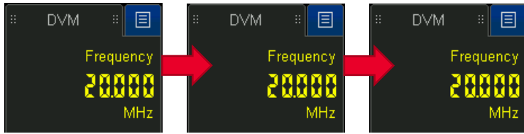
Figure 33. The precise 10-digit counter found the true frequency of a clock to be a little less than 20 MHz.
