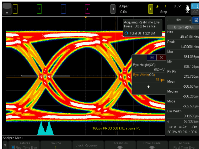
Figure 21. A real-time eye diagram measurement of a jittery 1-Gbps PRBS embedded clock signal. The histogram indicates a bimodal distribution and measured about 55-ps rms jitter.
