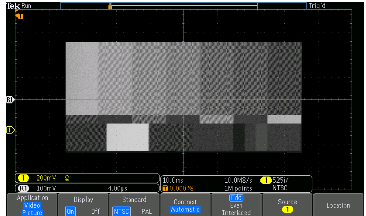
Viewing an NTSC full color bar signal image. Video picture mode contains automatic contrast and brightness settings as well as manual controls.
