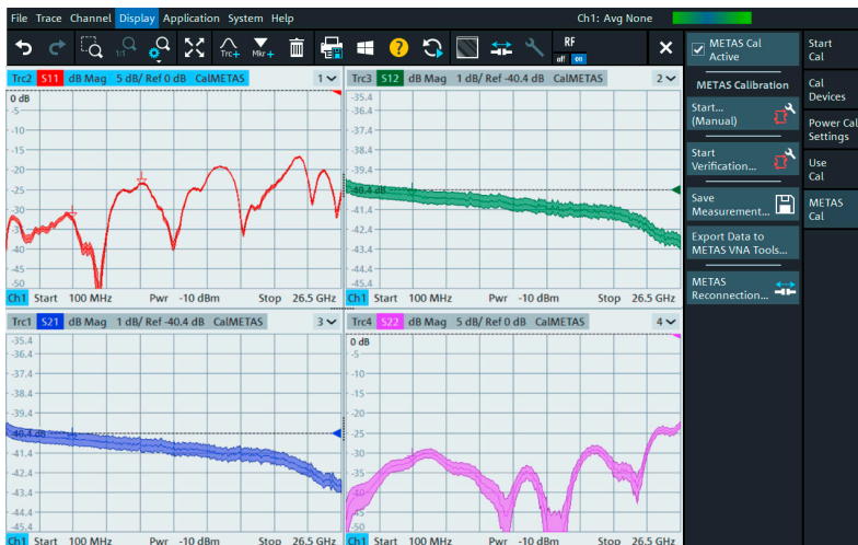
Real-time S-parameter measurements with uncertainty bands.
