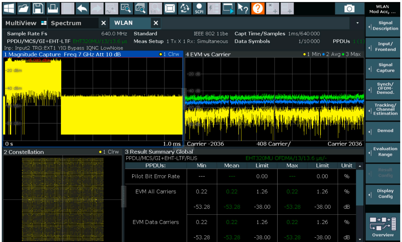
EVM measurement of an IEEE 802.11be signal with 320 MHz signal bandwidth
