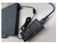
4. Power is being supplied from the electrical outlet to the AC adapter and onto your computer. Now, you are ready to turn on the computer.
