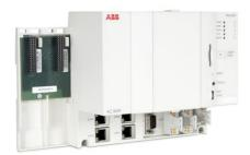
This CPU module is the medium base unit of the Freelance AC 900F controller family. It typically supports up to 1500 I/O and 8 MB battery buffered SRAM. 4 Ethernet interfaces, 800 MHz CPU clock, 24 MB Controller Memory, 8 MB battery buffered SRAM, and 16 MB DRAM. 2 slots for assembling Communication Interface Modules.
