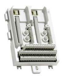
The TU842 MTU can have up to 16 I/O channels and 2+2 process voltage connections. Each channel has two I/O connections and one ZP connection. The maximum rated voltage is 50 V and maximum rated current is 3 A per channel.
