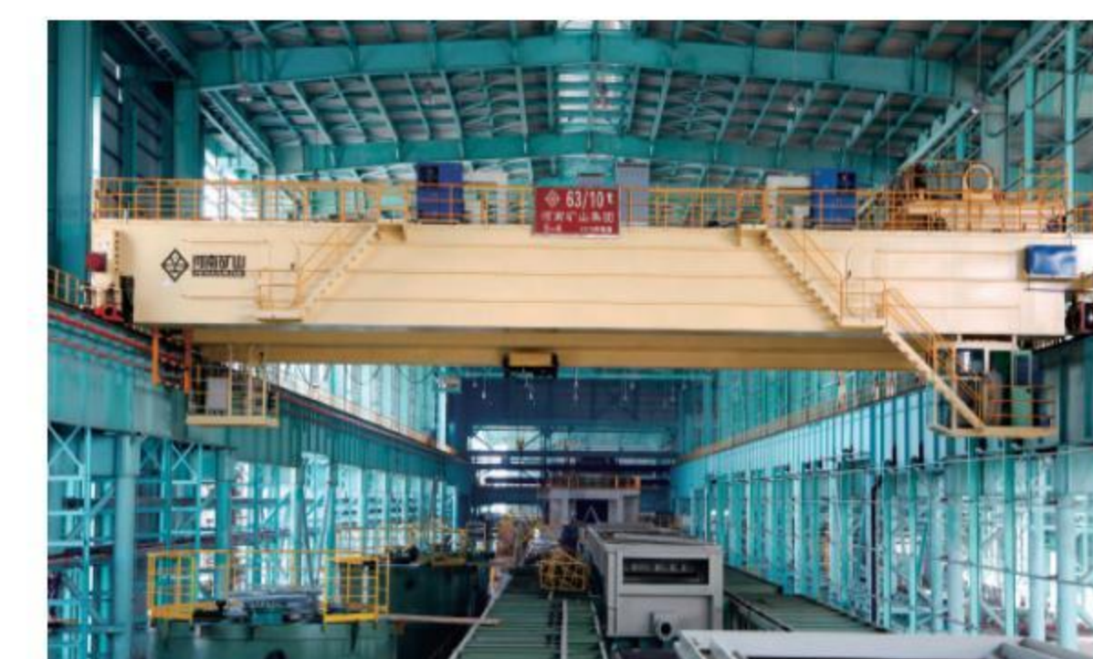
QD型电动双梁吊钩桥式起重机 QD type electric double beam bridge crane hook
