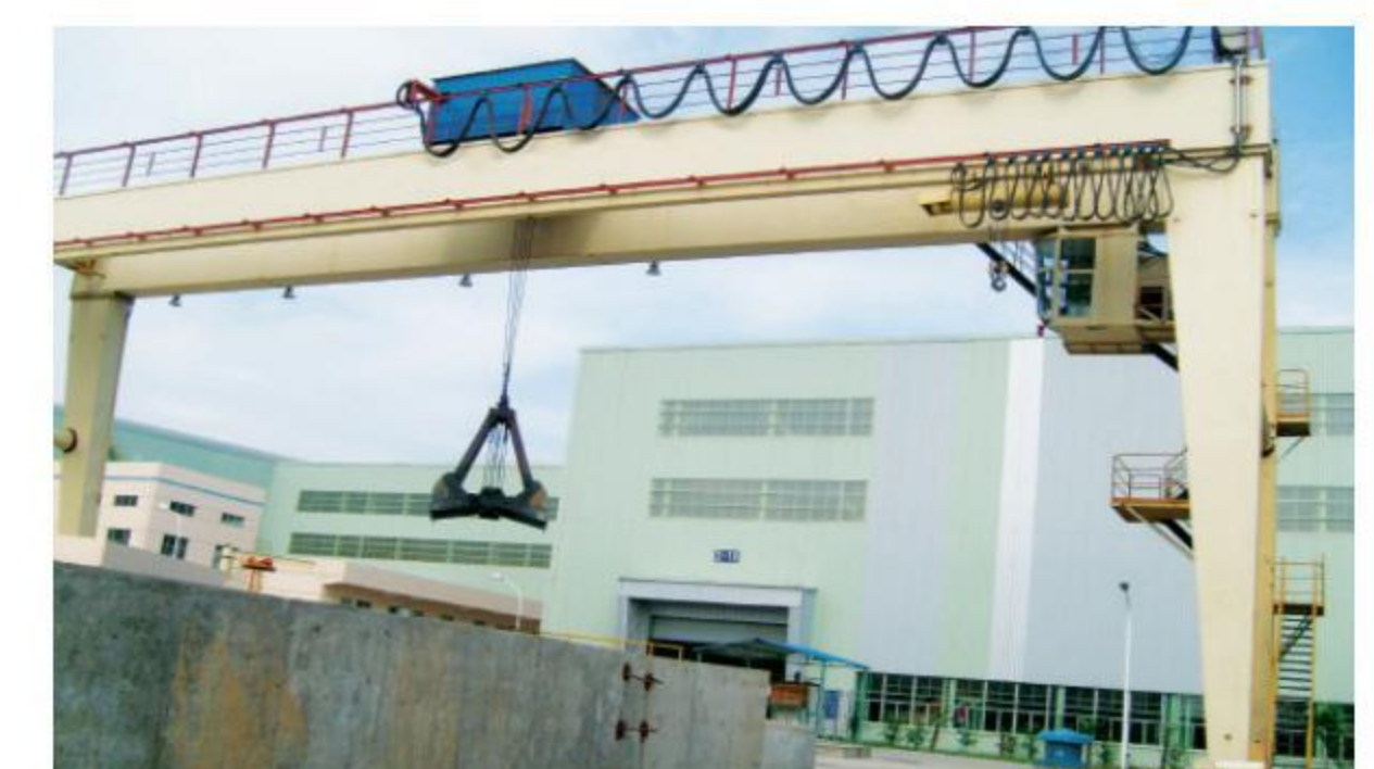
MZ型双梁抓斗门式起重机 MZ double beam grab gantry crane
