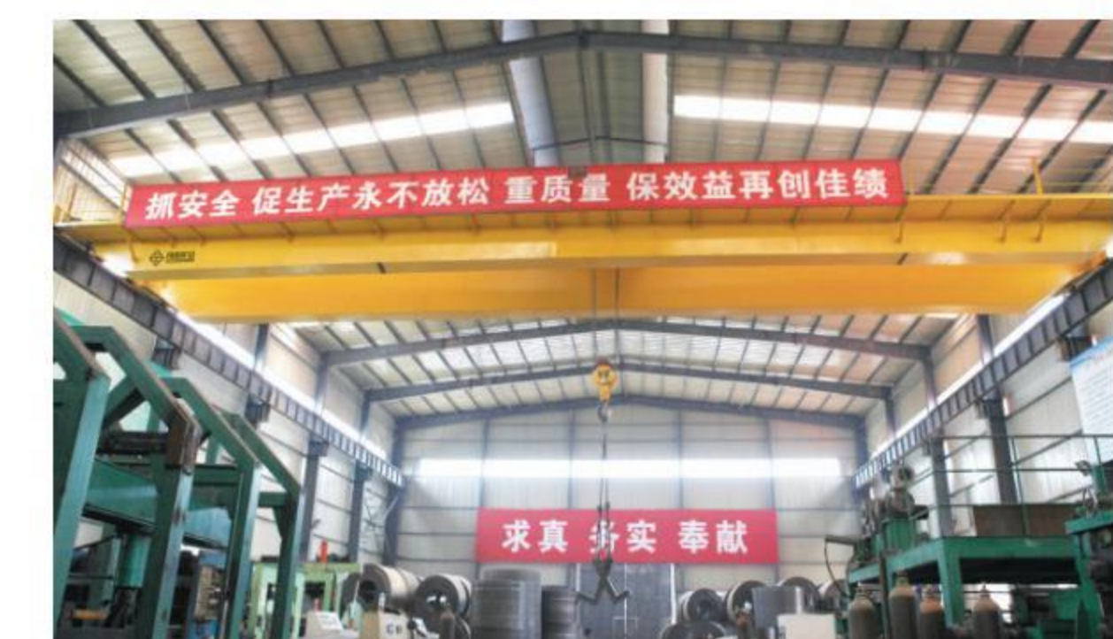
LH型电动葫芦双梁起重机 LH double-girder crane with electric hoist
