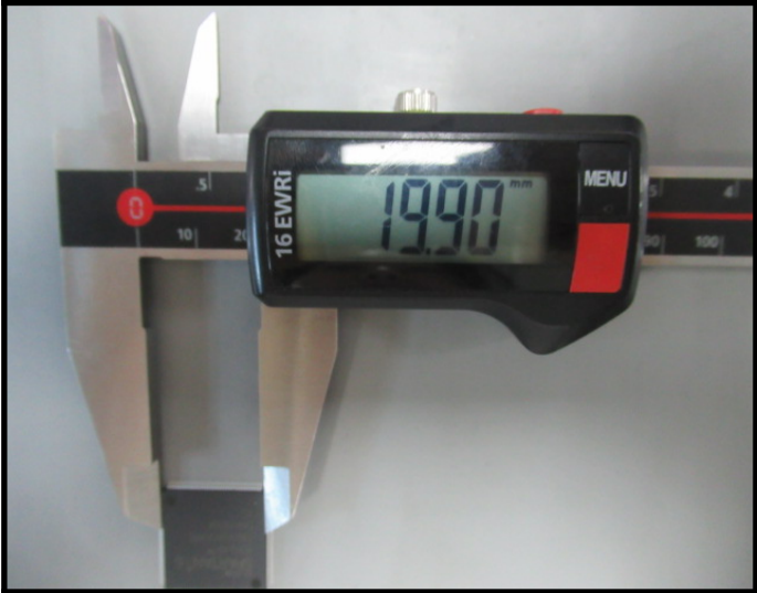
Dimension Measurement E1=19.90mm
