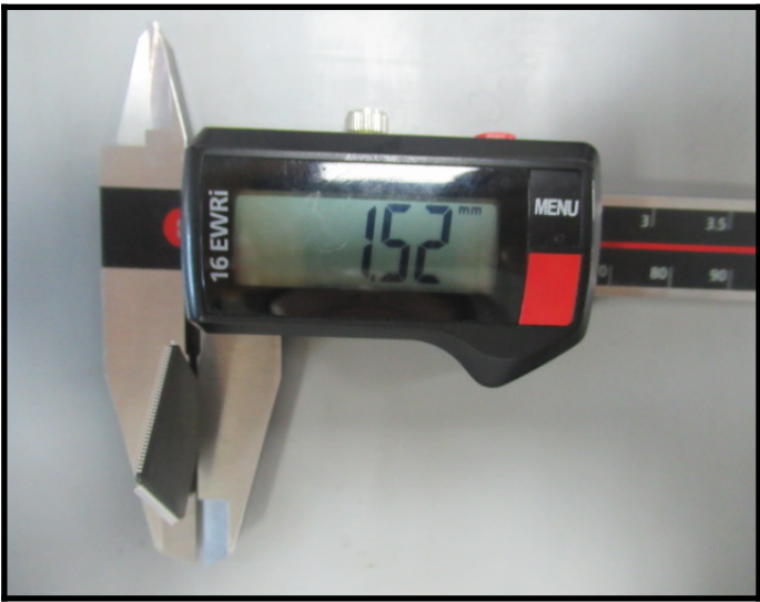
Dimension Measurement A=1.52mm (Pass)
