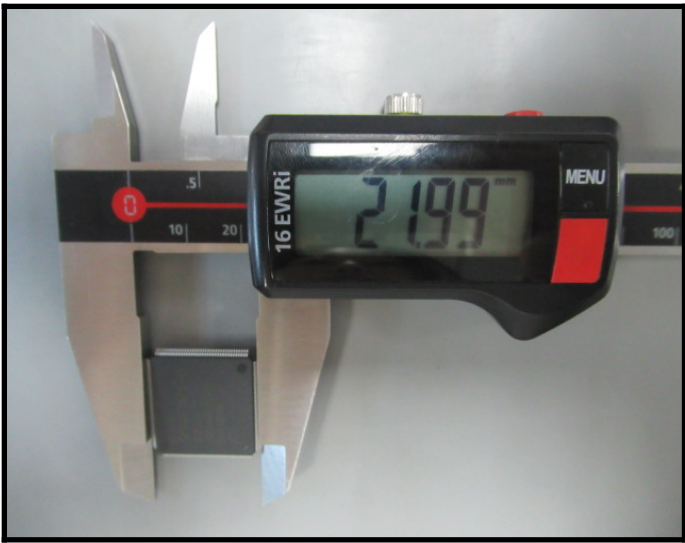
Dimension Measurement E=21.99mm
