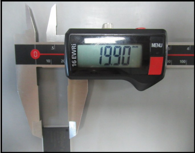
Dimension Measurement D1=19.90mm
