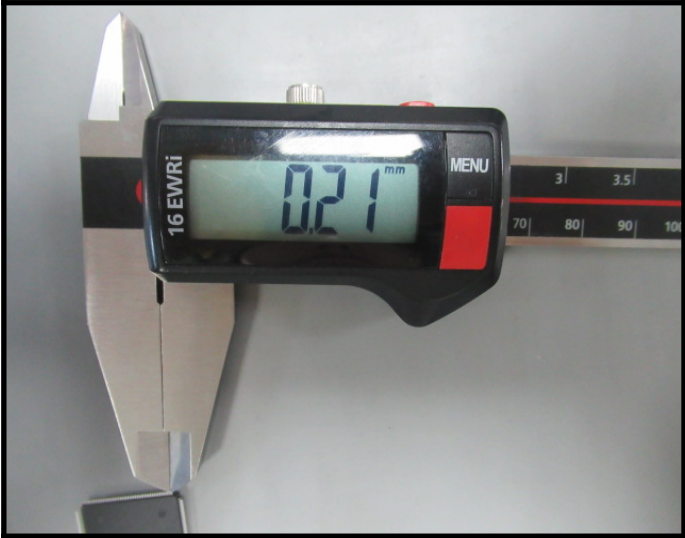
Dimension Measurement b=0.21mm (Pass)
