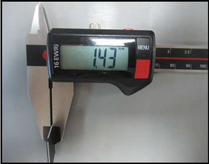
Dimension Measurement A2=1.43mm (Pass)
