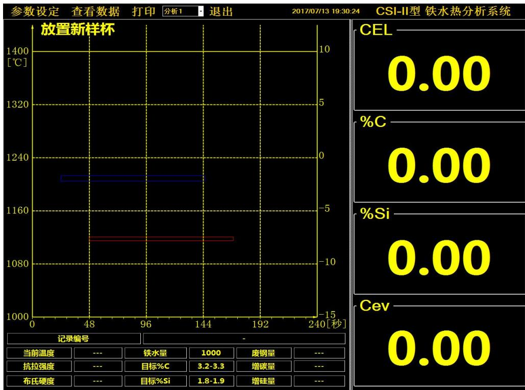
(2) After inserting the sample cup, the display shows (Ready to measure).
