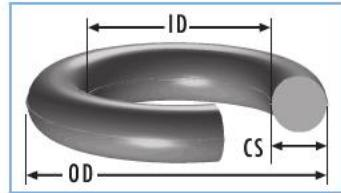
The sizes in the standard are defined by maximum and minimum ID and CS dimensions (although most listings, including this one, show this as a midpoint and a  $\pm$  tolerance). Each ID and CS combination is identified by a three-digit "dash number" as shown below.
