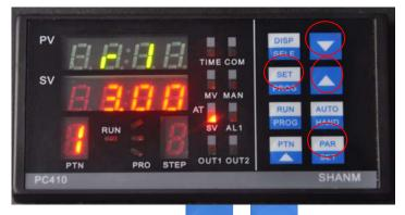
3) L1means the first seted temoweature, press can increase and decrease the fgure, we set165, press set to continue.
