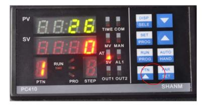
2) press PROG key to set the curve, r1means the first temperature rate, 3.00means Heating up 3 degrees per second
