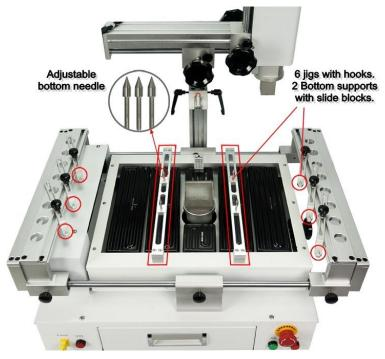
3. Increase the area of the bottom infrared heating plate, the size reaches 350\*250mm
