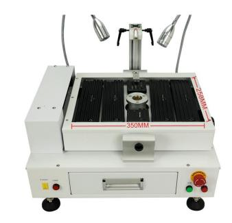
5. Lower infrared independent heating control switch for independent control of infrared heating plate
