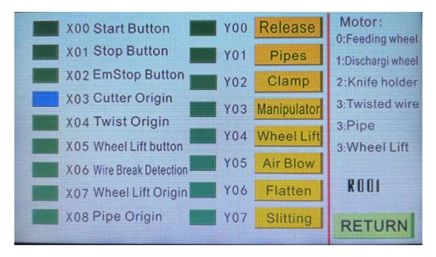
Each IO monitoring point corresponds to each wiring point of the main board. Usually, the monitoring is turned on when the machine is abnormal to determine the problem.
