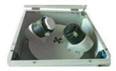
*Step4*: Cover machine cover and lock machine lock.
