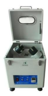
*Step2*: Take solder cream and put lining (remarks: don't need to add lining if solder cream diameter is more than  $\varphi$ 64.), take attached balance weights 500g.
