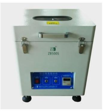
*Step5*: Set reference of mixing time at 15 minutes (remarks: H-hours, M-minutes, S-seconds in time relay), set to 15M00.
