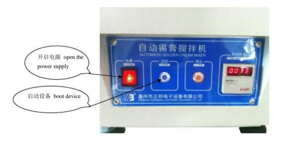
*Step7*: When mixing time is over and mixing head stops rotating, press stop button, turn the power off and remove the solder cream.
